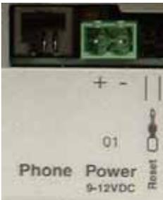
Remove reset jumper to enable power up of the Scout
